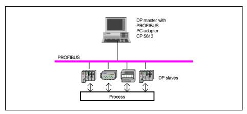
Figure 1 Basic Structure of a DP System.
