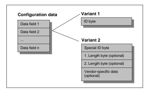
The two data block variants can be distinguished by bits 4 and 5 of the first byte.
